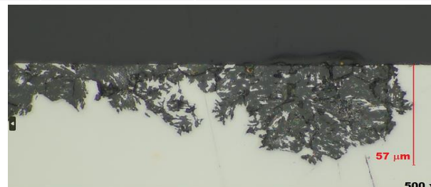
S13Cr deepest crevice (57 µm) characterization
