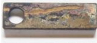
Mass loss/pitting coupon
