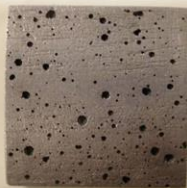
Mass loss/pitting coupon
